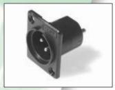
ACM 3 Pin chassis mounting Male XLR with counter sunk mounting holes for M3 screw fixing. XACM has non counter sunk mounting holes for self-tap screw fixing. Nickel Silver plated Brass contacts.
