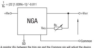
A resistor ( $R_{\rm U}$ ) between the trim pin and the Common pin will adjust the device output from +5V to +5.5V.
