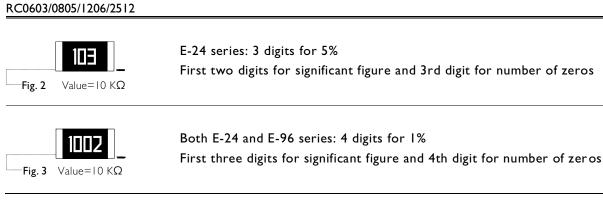
For further marking information, please refer to specific data sheet "Chip resistors marking".
