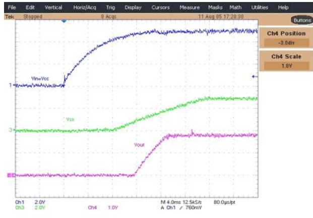
Figure 15 - Start up waveforms Ch1:Vin=Vcc, Ch3:Vss, Ch4:Vout
