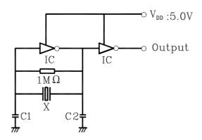
IC: 1/6TC4069UBP×2X: CERAMIC RESONATORC1 C2: 30pF +/-20%
